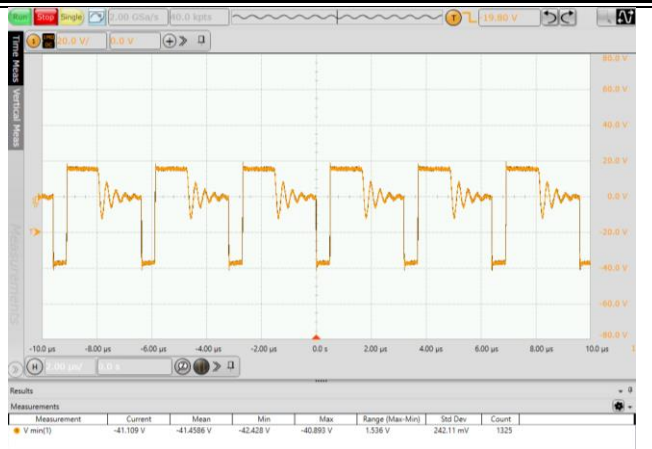
Fig. 5.10 Secondary-side output diode stress waveform (VIN=36V, 100% Load)
