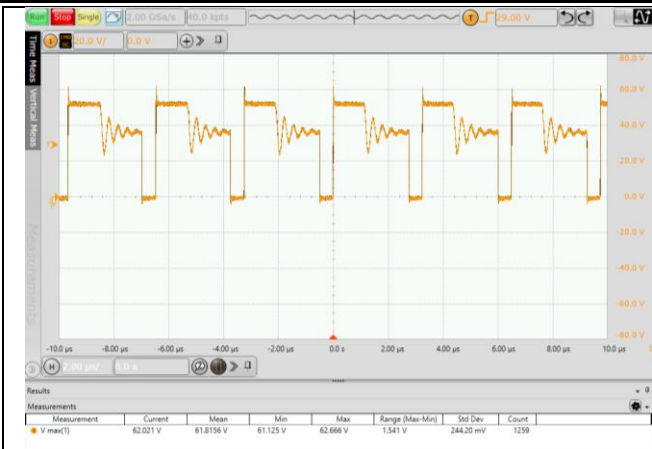
Fig. 5.9 MOS Voltage stress waveform (VIN=36V, 100% Load)
