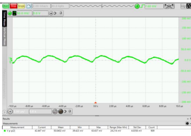
Fig. 5.6 Output voltage ripple waveform (VIN=24V, 100% Load)
