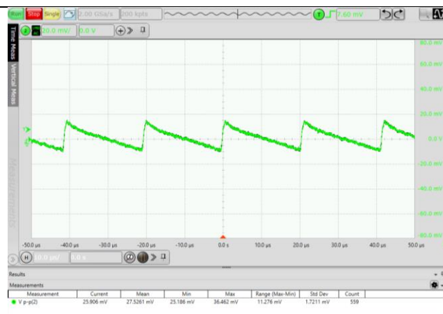
Fig. 5.5 Output voltage ripple waveform (VIN=24V, 5% Load)
