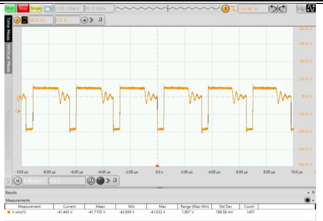
Fig. 5.10 Secondary-side output diode stress waveform (VIN=36V, 100% Load)
