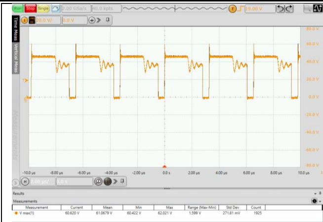
Fig. 5.9 MOS Voltage stress waveform (VIN=36V, 100% Load)
