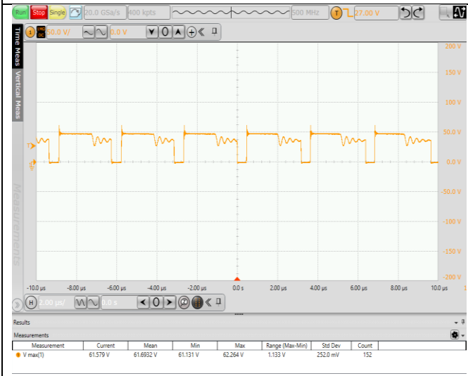
Fig. 5.9 MOS Voltage stress waveform (VIN=36V, 100% Load)
