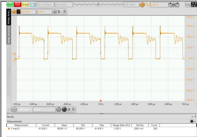
Fig. 5.9 MOS Voltage stress waveform (VIN=36V, 100% Load)
