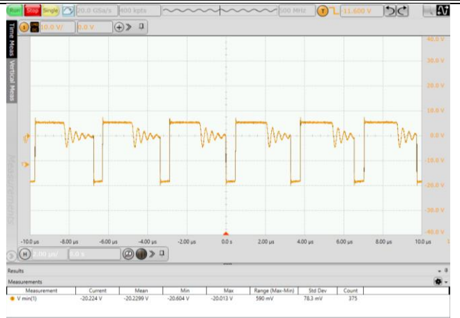
Fig. 5.10 Secondary-side output diode stress waveform (VIN=36V, 100% Load)
