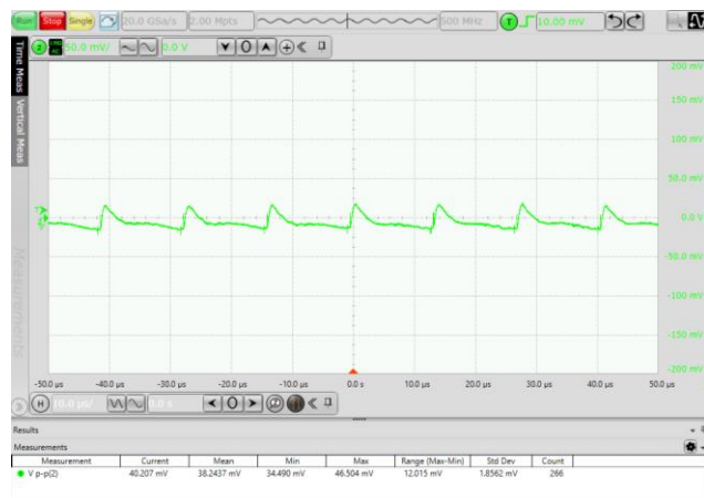
Fig. 5.9 Output voltage ripple waveform (VIN=24V, 5% Load)
