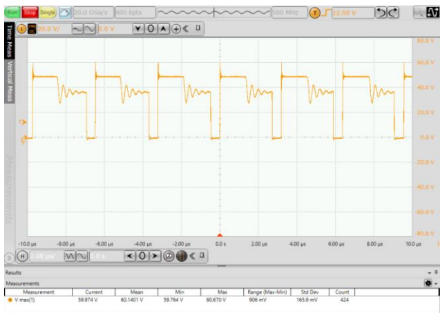
Fig. 5.13 MOS Voltage stress waveform (VIN=36V, 100% Load)
