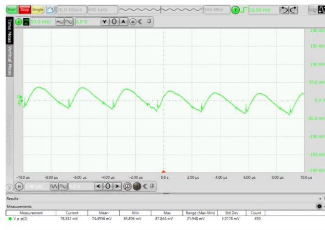
Fig. 5.10 Output voltage ripple waveform (VIN=24V, 100% Load)
