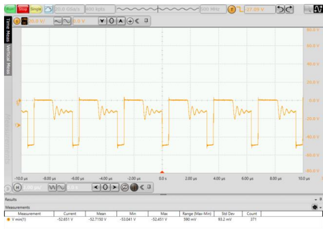
Fig. 5.14 Secondary-side output diode stress waveform (VIN=36V, 100% Load)
