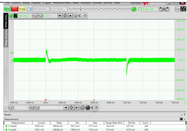
Fig. 5.7 25% -50% -25%IO Dynamic waveform (VIN=24V)
