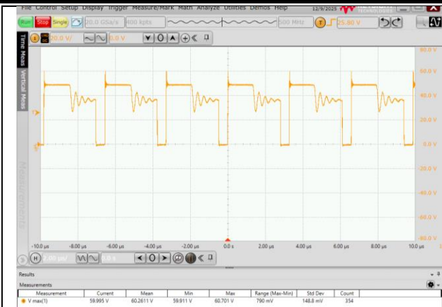
Fig. 5.9 MOS Voltage stress waveform (VIN=36V, 100% Load)
