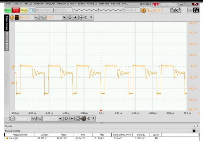
Fig. 5.10 Secondary-side output diode stress waveform (VIN=36V, 100% Load)
