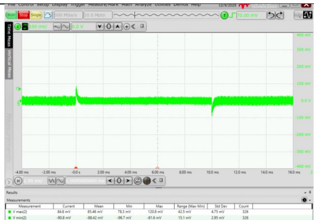
Fig. 5.6 Output voltage ripple waveform (VIN=24V, 100% Load)
