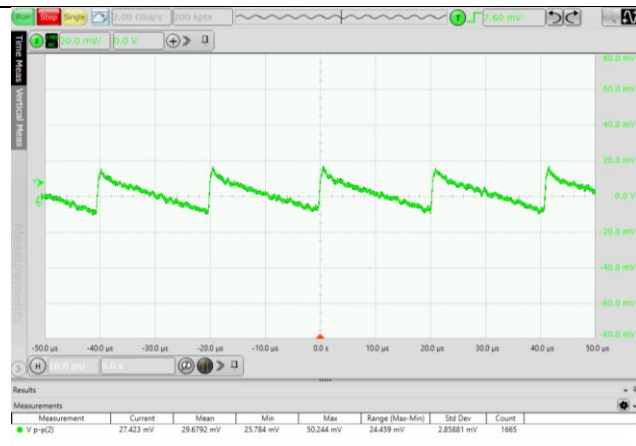
Fig. 5.5 Output voltage ripple waveform (VIN=24V, 5% Load)
