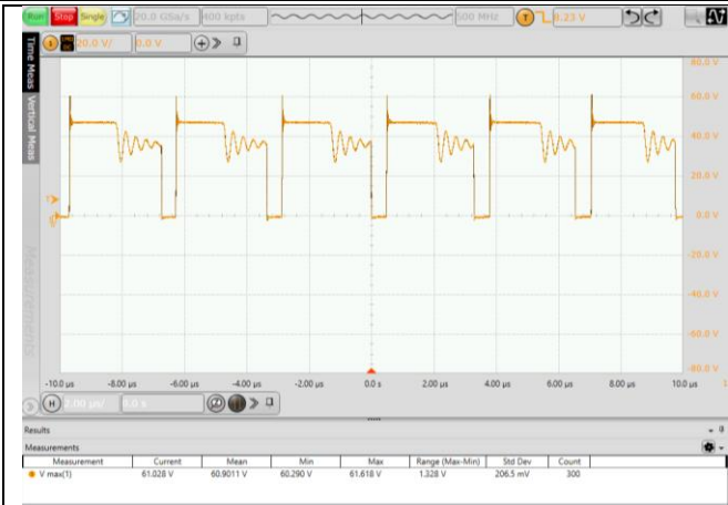
Fig. 5.9 MOS Voltage stress waveform (VIN=36V, 100% Load)
