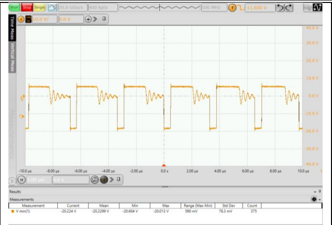
Fig. 5.10 Secondary-side output diode stress waveform (VIN=36V, 100% Load)
